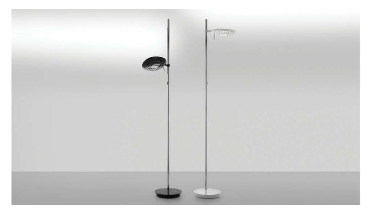
A single latest-generation LED light source of just 40W guarantees the same illuminance values that are obtainable with a 400W halogen. Visual lightness and thermodynamics are the main characteristics of the project: the head, made of die-cast aluminium, is appropriately shaped and perforated to form a permeable visual interface for the space where it is placed and facilitates heat exchange, guaranteeeing optimum dissipation of the heat produced by the light source
